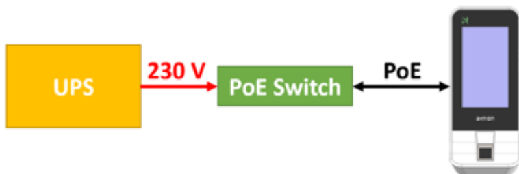
Obr. 6: PoE switch s UPS
