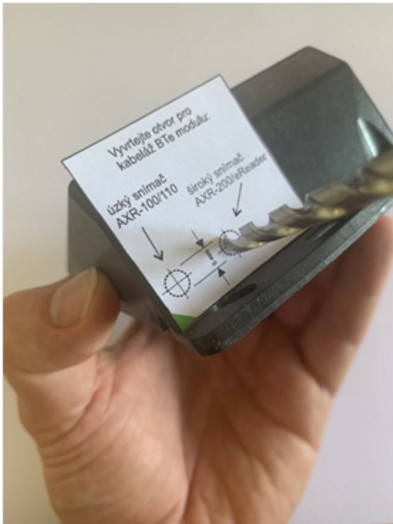
Fig. Drilling the hole for the wide casing (ER, AXR-2xx) (AXR-1xx)
