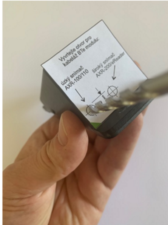
Fig. Drilling a hole for a narrow casing
