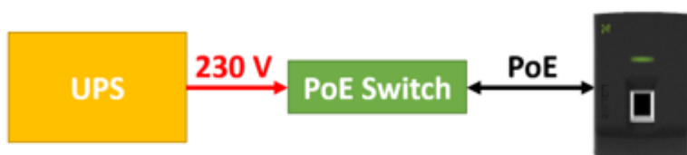
Obr. 5: PoE switch s UPS
